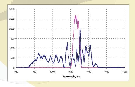
Spectra and autocorrelation traces: purple curves – output pulse of ytterbium laser with duration of 290 fs, blue curves – after spectral broadening in a capillary filled with Xe and subsequent compression down to 27 fs.
